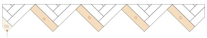
Measuring the L1 plank cut-off.
