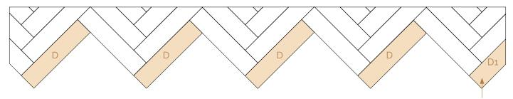
Measuring the R1 plank cut-off – repeat the same procedure as for the L1 plank.
